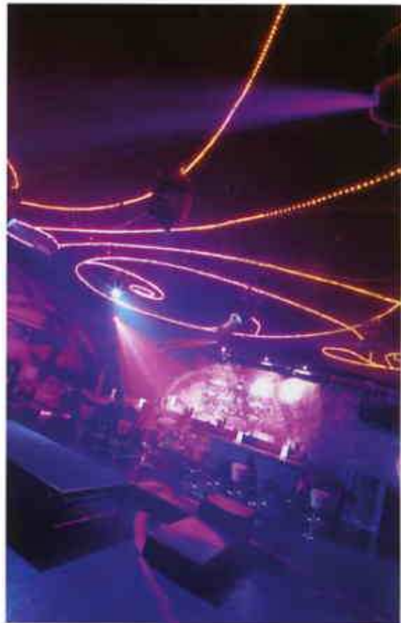
Top: the white external walls of Momo are washed with Studio Due Mini City colour changers. Above: the butterfly rig in the main dance room is illuminated by rope lighting and hung with Martin Pro fixtures
