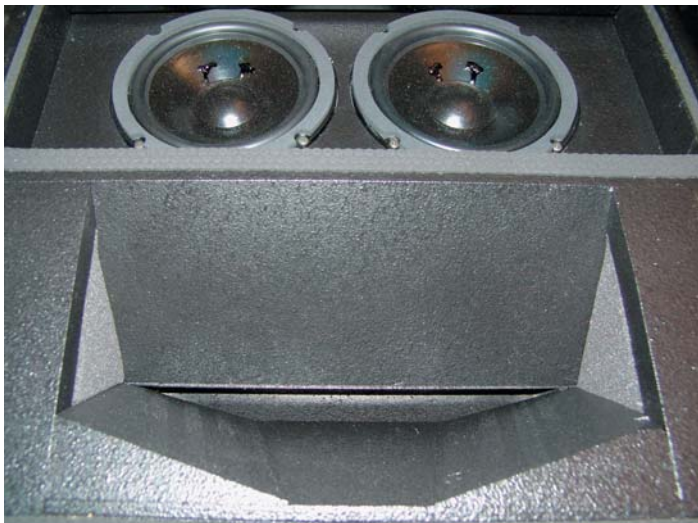
The Horn uses a parabolic reflector and a wide diffraction slot which acts like a large ribbon tweeter. The basic construction of this waveguide is shown in the illustration below using the H.A.R.D 212 monitor as an example.
